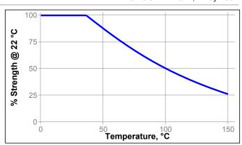
**Heat Aging** Aged at temperature indicated and tested @ 22 °C
