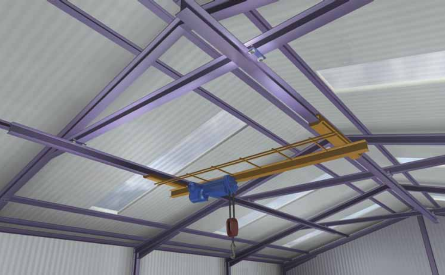
Installation of a new runway beam for a crane
