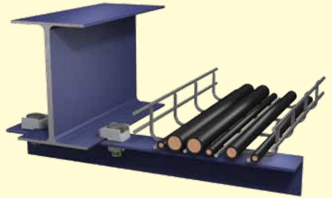
Cantilevered angle support for running cable tray
