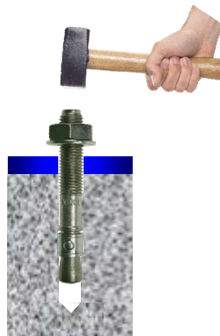
Insert assembled anchor through fixture into concrete
