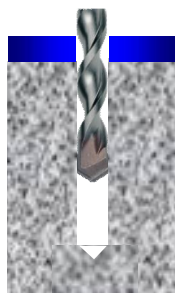
Position fixture and drill correct diameter hole to correct depth
