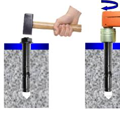
Insert assembled anchor through fixture into concrete Tighten with torque wrench to recommended torque
