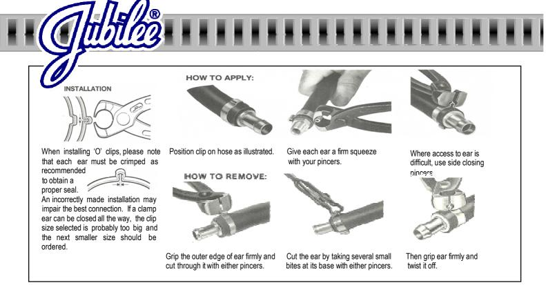
While both ears must be closed all the way to effect a proper seal, 2-ear clamps are best installed with one ear closed all the way first. The second ear is then closed so that the first ear opens slightly (gap to be approximately 1.5mm). This builds a resilient strength into the clamp in a spring-like action to hold against pressure, vibration and hose shrinkage due to temperature changes or ageing.
